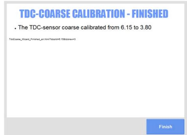
Use this sequence only as an emergency. The coarse calibration should only be done during the segment change or a TDC sensor exchange.
