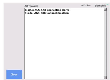
The Service form will indicate alarms for the missing functions in the AGS head.
